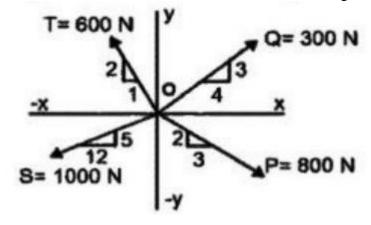
2. Coplanar concurrent forces are acting at a point as shown in fig. Find the 1 UN 16 magnitude and direction of the resultant.
