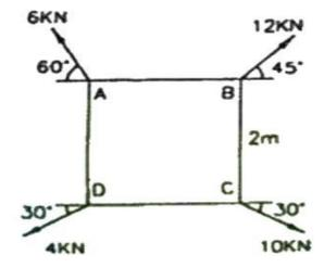
5. Calculate the resultant force and its direction. For the Fig. shown
