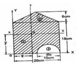
7. Find Moment of Inertia about the co-ordinate axes of plane area shown in 3 AP 16 fig.
