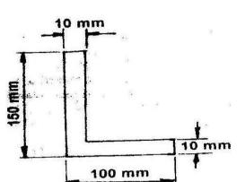
3. Locate the centroid of the area shown in figure below. The dimensions are 3 AP 16 in mm.
