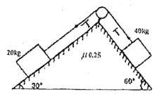
4. An inextensible string passing over a smooth pulley as shown in Fig. joining two blocks. If the blocks are released simultaneously from rest, determine the velocity of block A after it has moved over 2 m and the tension in the string. Assume the co-efficient of friction at the contact surface is 0.2. Use energy principle.
