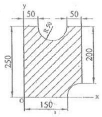
5. Find the moment of inertia of the centroidal axes for the section shown in fig.
