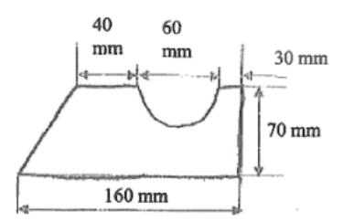
6. Locate the centroid of the shaded area shown in fig. The dimensions are in 3 AP 16 mm.
