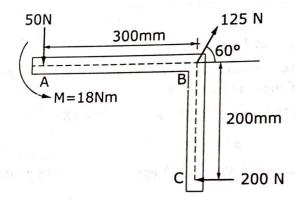
7. Determine the support reactions of the beam as shown in fig.
